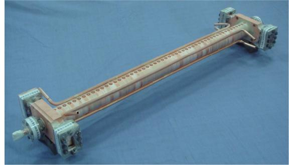
Figure 10: The model for high power RF test.
