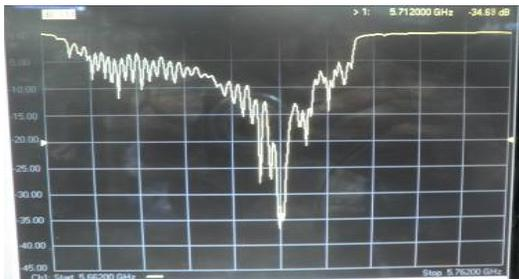
Figure 8: The S11 characteristic of full band (100MHz).
