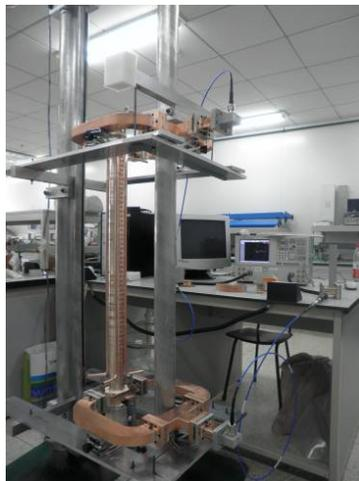
Figure 4: The vertical setup for C-band accelerating structure RF cold test.
