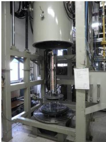
Figure 3: The structure brazing in the hydrogen furnace.
