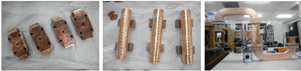
Figure 2: Components of C-band accelerating structure.
