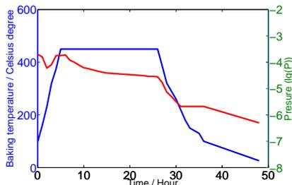
Figure 9: Vacuum level and temperature during baking
