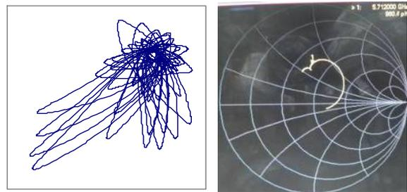
Figure 5: The mismatch status of accelerating structure Left: field distribution on axis; Right: S11.
