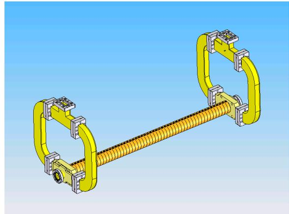
Figure 1: The drawing of the C-band accelerating structure.
