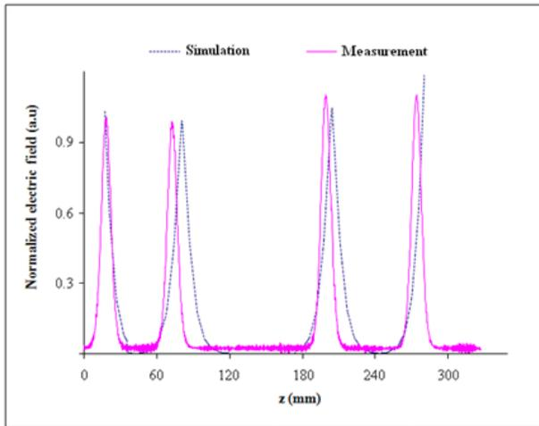
Figure 2: Field distribution in the cavity
