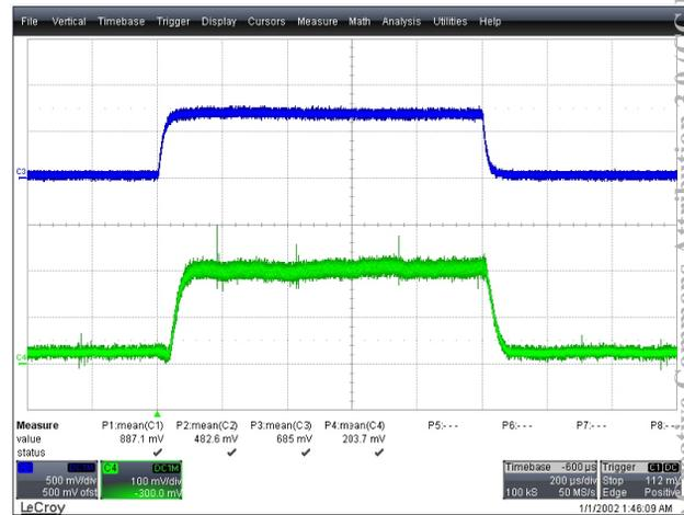
Figure 4a: Forward power (C3) and beam current (C4) signals.
