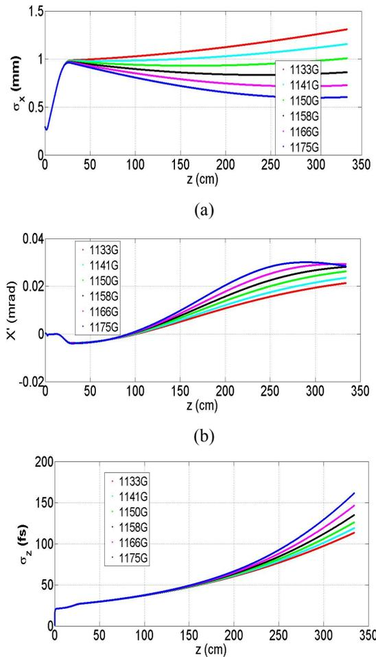
Figure 5: Simulation result with the single cell RF gun. (a)  $X_{rms}$  vs  $z$  (b) Divergence vs  $z$  (c) Bunch length vs  $z$
