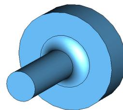
Figure 2: Schematic 3D view of single cell RF gun for FED.
