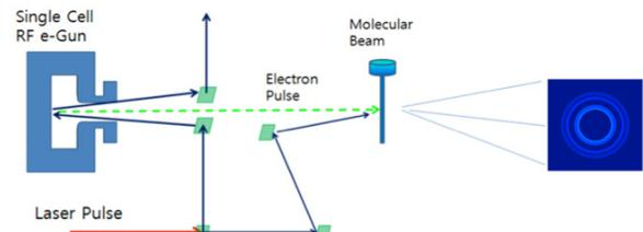
Figure 1: Schematic setup of the FED experiment with single cell RF gun.
