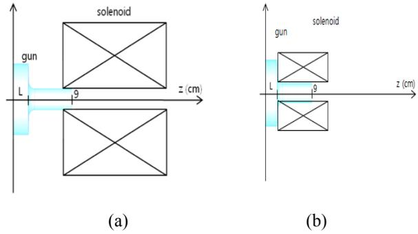
Figure 4: (a) Schematic view of simulation configuration used in this study (b) Future plan of the solenoid design
