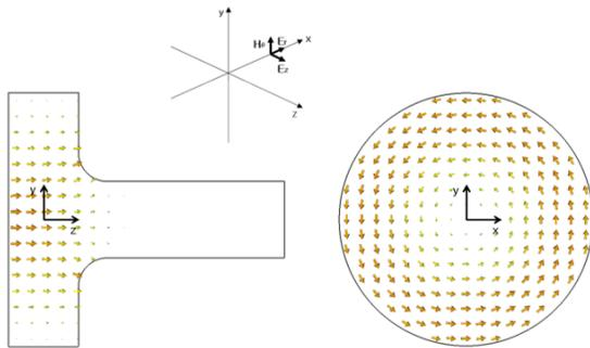
Figure 3. (a) Side view of single cell RF gun with electric field distribution. The direction of arrows is the direction of electric field in the gun. The length of arrows is the amplitude of the E-field. (b) The front view of the rf gun with magnetic field in the gun.
