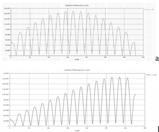
Figure 9: Distribution of E-field along of the longitudinal axis (a) –without optimization, (b) – with cutted planes
