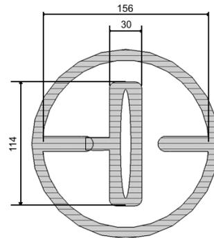
Figure 10: IH-resonator with vertically placed drift tubes and thickened electrodes.
