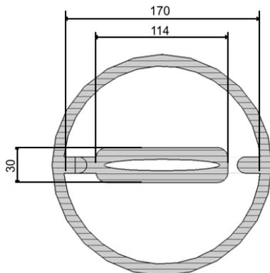
Figure 4: Horizontally placed drift tubes into IH-resonator with thickened electrodes.
