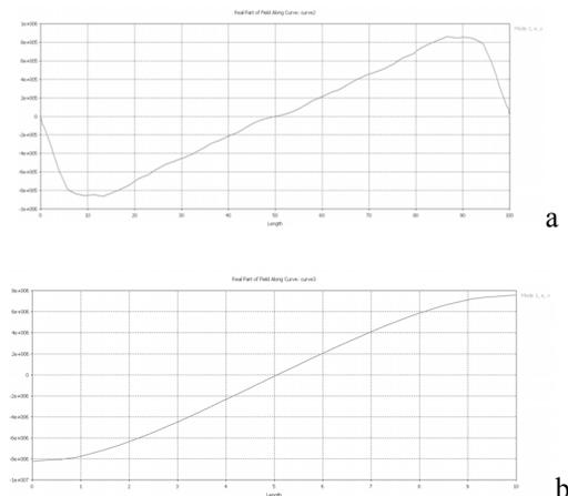
Figure 11: Resonator with vertically placed tubes distributions: electric field within drift tubes (a) – vertical axis, (b) – horizontal axis.
