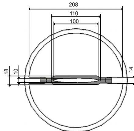
Figure 1: IH resonator with horizontally placed drift tubes. Front view.
