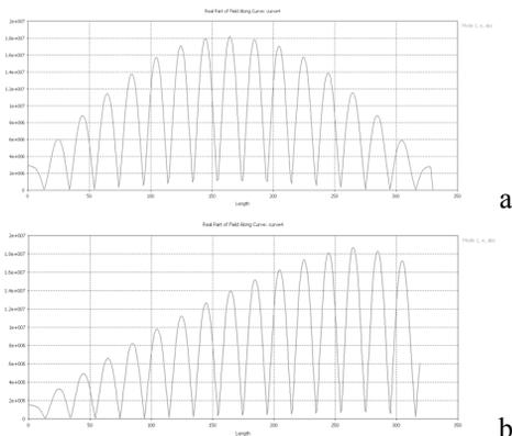
Figure 3: Distribution of E-field on longitudinal axis in resonator with horizontally placed drift tubes (a) – without optimization, (b) – with cutted planes.
