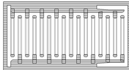
Figure 2: IH resonator with horizontally placed drift tubes and vanes cutting. Top view.
