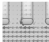
Figure 7: Distortion of magnetic field around vertically placed drift tubes.
