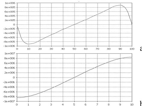
Figure 5: Resonator with horizontally placed tubes distributions: electric field within drift tubes (a) – horizontal axis, (b) – vertical axis.
