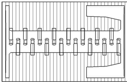
Figure 8: IH-resonator with vertically placed drift tubes and vanes cutouts. Top view.
