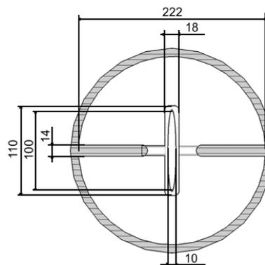
Figure 6: IH-resonator with vertically placed drift tubes.
