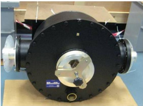
Figure 3: CaCo, a Cavity Combiner.
