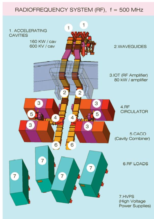
Figure 1: Two RF plants in one straight section.
