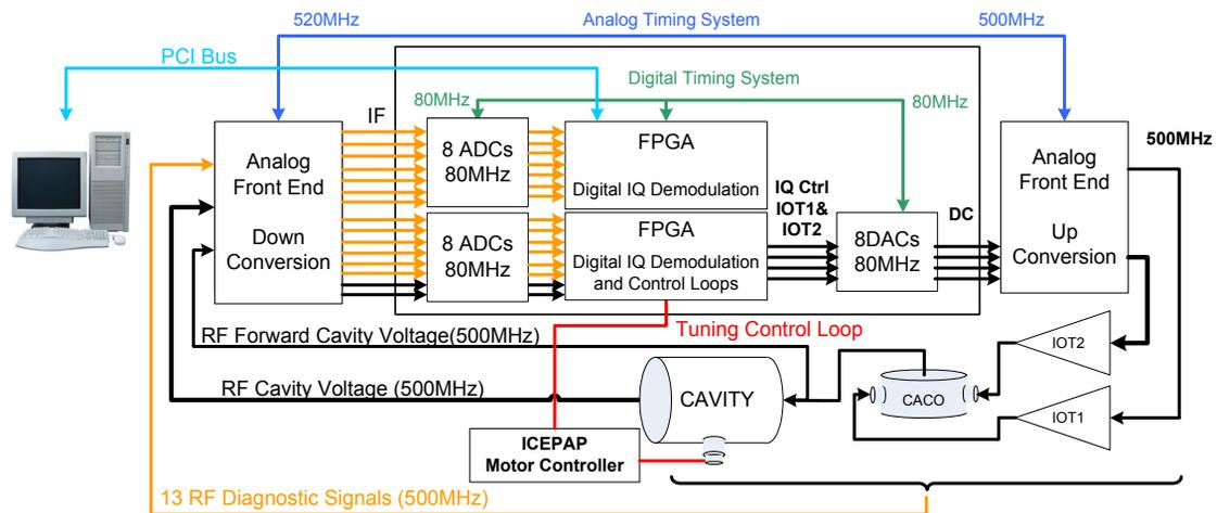
Figure 5: Digital LLRF Hardware Scheme.
