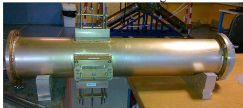
Figure 7: Picture of the CoStub to short cut the coaxial line of the IOT arms.
