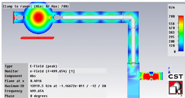
Figure 5: Simulation of the standing wave in the passive IOT arm.
