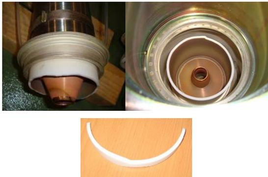
Figure 3: Broken IOT in three parts.
