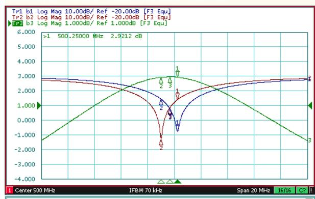
Figure 2: CaCo response with a 10° phase difference at the input ports.
