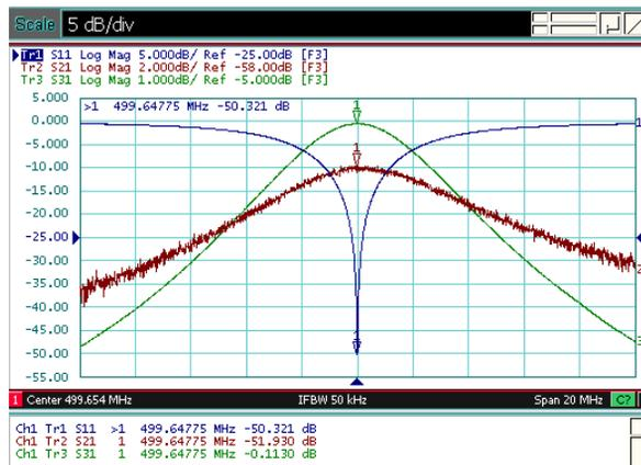
Figure 9: CoStub S-parameters showing complete isolation of the passive IOT.
