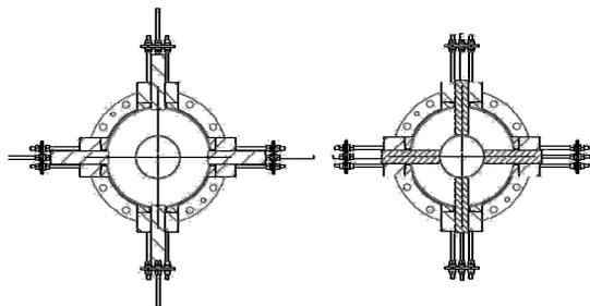
Figure 8: Cross section of the CoStub in symmetrical (left) and asymmetrical (right) modes.
