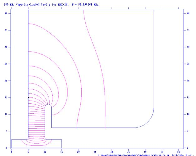
Figure 1: Main cavity profile.
