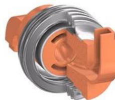
Figure 10: 3D model of the double-sector choke flange.
