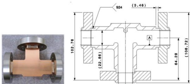
Figure 6: X-band splitter
