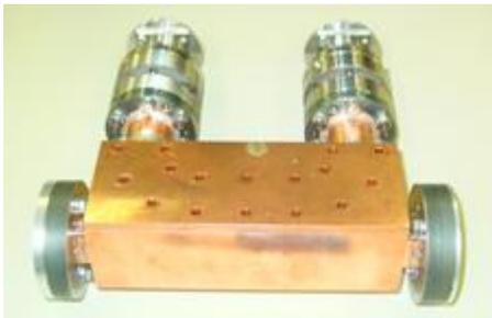
Figure 3: Bi-directional coupler by GYCOM Ltd
