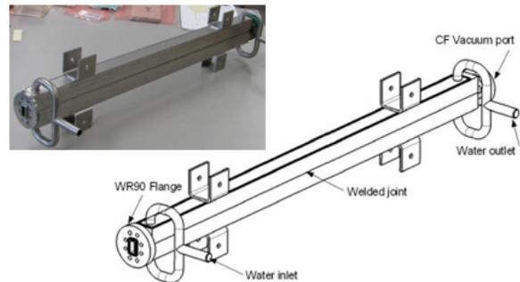
Figure 1: 3D model of X-band high power load
