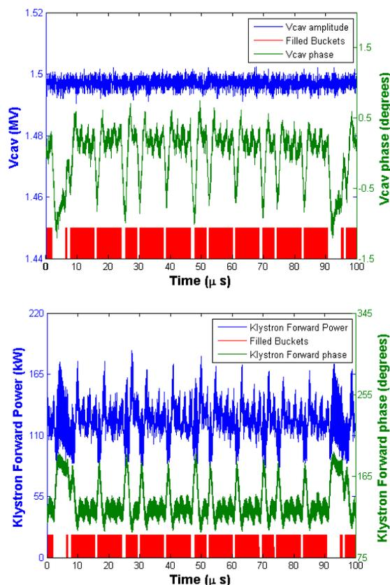
Figure 4: Cavity field (top) and klystron drive (bottom) in physics conditions. Beam current in red. The revolution period is 88.9  $\mu$ s.
