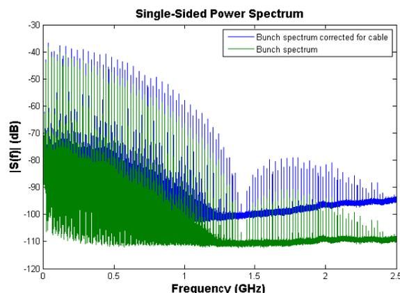
Figure 2: Beam current spectrum with 1380 bunches, without and with compensation for cable response.
