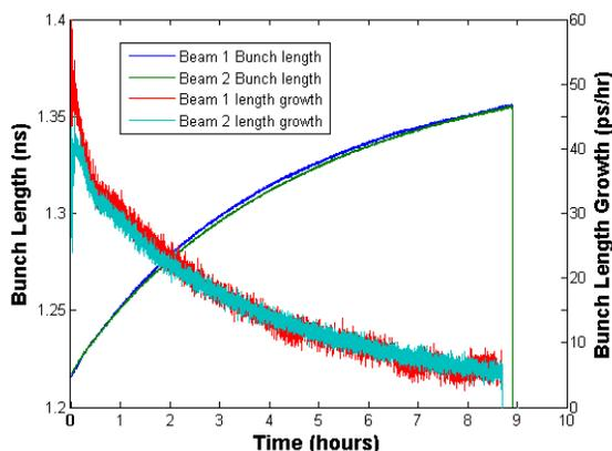
Figure 3: Evolution of bunch length mean and growth rate during physics. 1380 b/beam,  $1.3 \times 10^{11}$  p/bunch.
