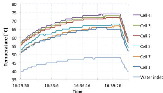
Figure 3: Temperatures measured at the outside of the PIMS cavity (at the center of the ring). The sensor of the cell 6 was detached during the test. The water temperature of the cooling water inlet rose to 48°C. The order from top to bottom in the legend corresponds to the order in the plot.
