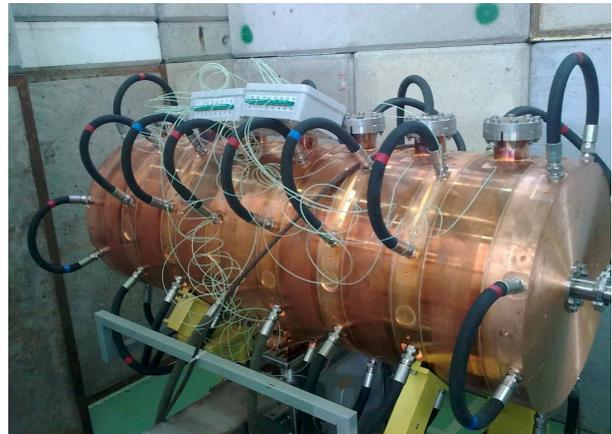
Figure 1: The PIMS cavity connected inside the bunker.
