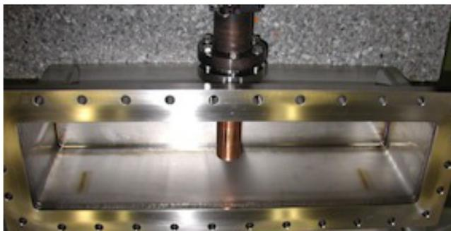
Figure 3: Prototype TaCo used for high-power tests
