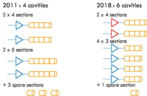
Figure 4: Proposal for cavity and power upgrade
