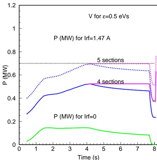
Figure 1: Power per SPS 200 MHz cavity having 4 or 5 sections for nominal and zero (green) beam current during the LHC cycle with two voltage programs (blue - voltage for constant filling factor in momentum for emittance of 0.5 eVs, red - constant 4.5 MV at the end of the cycle increased to 7.0 MV prior extraction to LHC).
