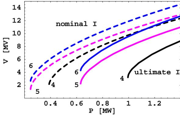
Figure 3: Total voltage possible for nominal and ultimate LHC intensity for different RF configurations from Table 2 with 4 (present situation), 5 or 6 cavities as a function of power limit per cavity.
