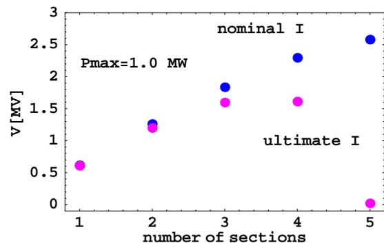
Figure 2: Voltage from one SPS 200 MHz TW cavity having different number of sections for nominal (top circles) and ultimate (bottom circles) beam current.
