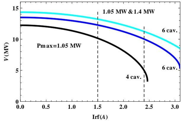
Figure 5: Total voltage possible on the flat top with 4 (present situation) and 6 cavities as a function of beam current for two options of power upgrade for 6 cavities (top curve - 1.05 MW per each 3-section cavity and 1.4 MW for each 4-section cavity; middle - 1.05 MW/cavity). Dashed lines are at nominal and ultimate beam currents.
