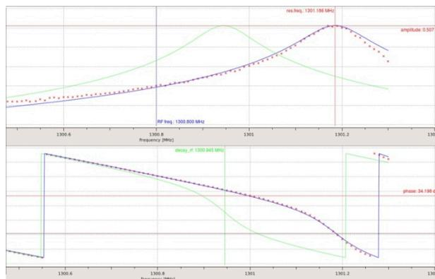
Figure 5: Red and Blue traces show the results of sweep analysis; Green is the current cavity frequency.
