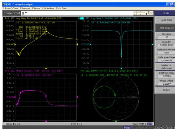
Figure 4: EMMA RF cavity response using VNA showing notch in response.
