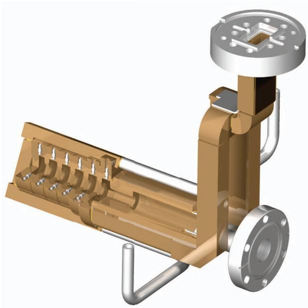
Figure 2: CAD rendering of Mark 1 X-band RF photoinjector.
