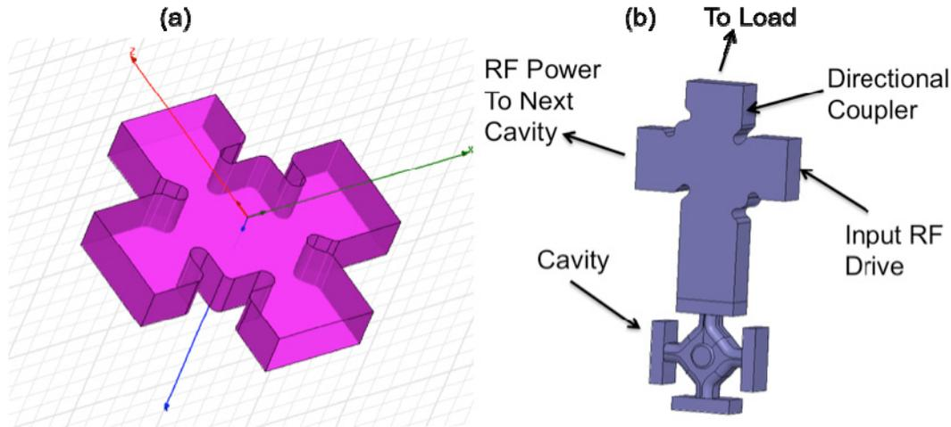
Figure 2: Biplanar coupler and cavity coupling configuration. (a) Internal structure of biplanar coupler. (b) Connection of biplanar coupler to one of the cavity ports.
