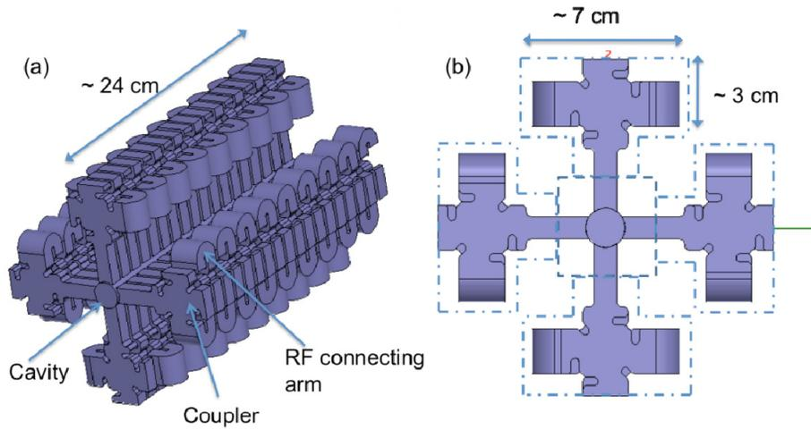
Figure 3: Conceptual schematic of rf feed system for a set of SW cavities.
