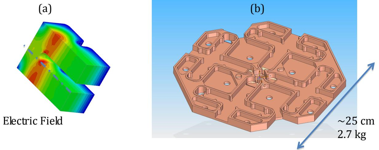
Figure 4: Planar construction of cell, couplers and connection arms. (a) Electric field in planar 180 degree elbow (plot is split at half guide width). (b) CAD design of cell plate.
