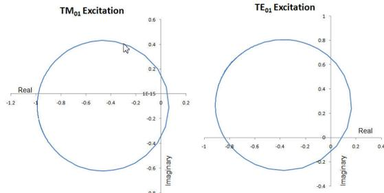
Figure 3: Smith chart from simulations showing each mode is slightly over-coupled
