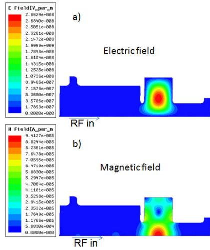
Figure 6: TE<sub>011</sub> electric and magnetic fields normalised to 10MW power loss. a) electric, b) magnetic
