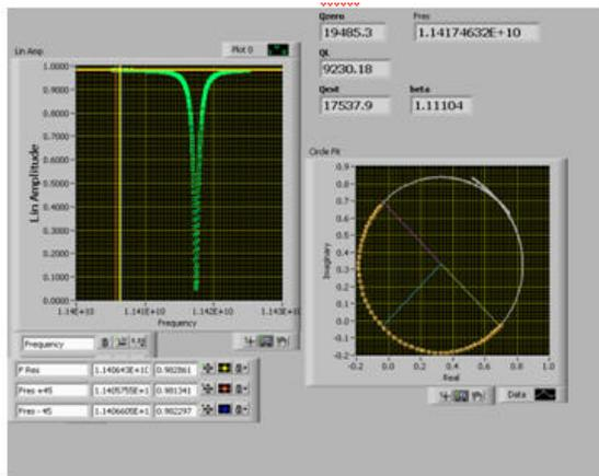
Figure 5: Cold Test measurements – TM<sub>020</sub> mode
