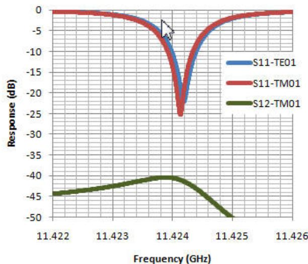
Figure 2: Simulated S-parameters for the  $TE_{011}$ - $TM_{020}$
