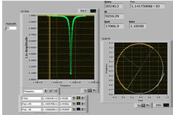
Figure 4: Cold Test measurements – TE<sub>011</sub> mode
