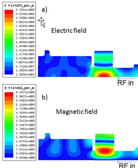
Figure 7: TM<sub>020</sub> electric and magnetic fields normalised to 10MW power loss. a) electric, b) magnetic
