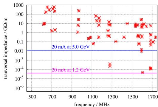
Figure 4: Transverse shunt impedances  $R_{\perp}$  of dipole HOM and typical threshold impedances for transverse CBI at a beam current of  $20 \text{ mA}$  at ELSA.
