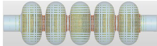
Figure 1: Elliptic geometry (cell length: 300 mm, cell diameter: 532.5 mm, beam pipe diameter: 202 mm) of the five-cell SC 500 MHz cavity with electric field distribution of the  $TM_{010}$   $\pi$ -mode for beam acceleration. Simulated with the eigenmode solver of CST Microwave Studio<sup>®</sup>.
