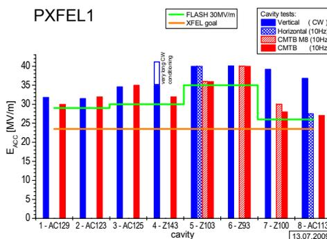
Figure 7: Cavities tests results for module PXFEL 1.
