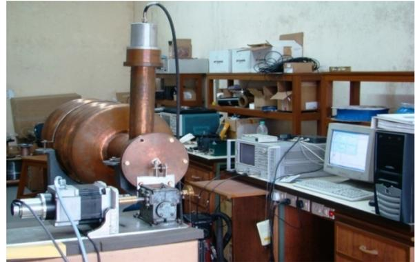
Figure 2: bead pull measurement set up for 5-cell elliptical shape copper prototype cavity.
