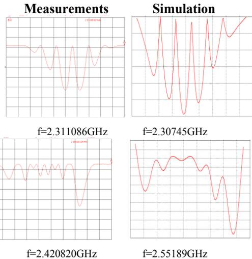
Figure 7: Comparison of some monopole HOMs in the cavity and the simulation
