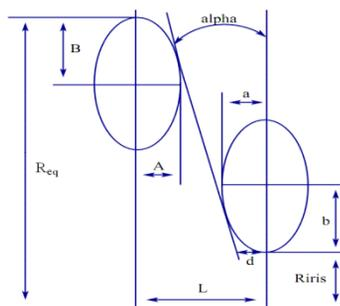
Figure 1: Geometry parameters for a half cell
