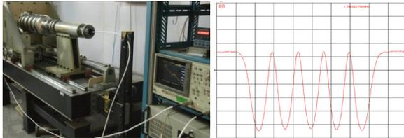
Figure 6: (a) tuning system at PKU (b) field flatness after tuning
