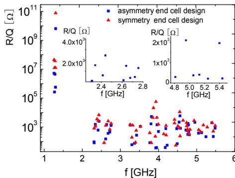
Figure 3: Spectrum of monopole mode
