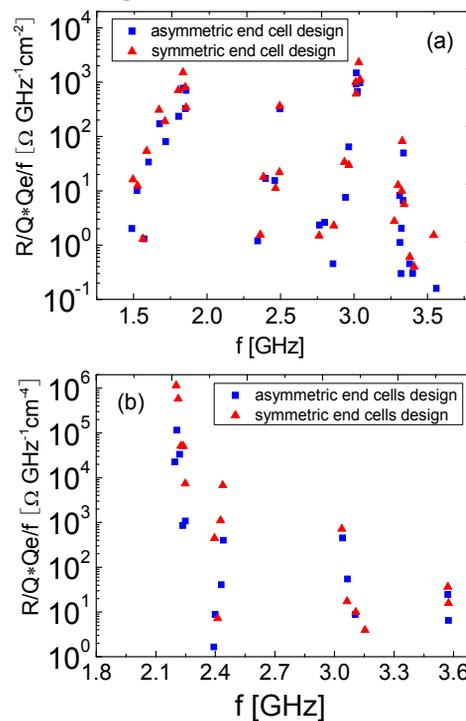
Figure 4: (a) Spectrum of the dipole HOMs, (b) Spectrum of the quadrupole HOMs
