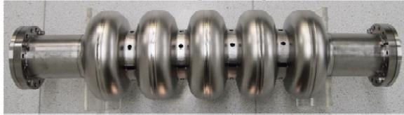
Figure 5: 5-cell niobium high current cavity
