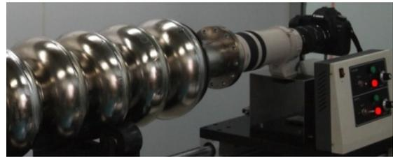
Figure 8: Optical inspection system at PKU
