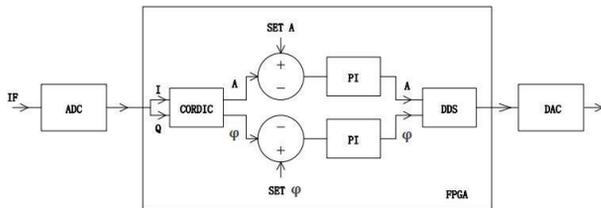
Figure 3: Internal Algorithm of FPGA.
