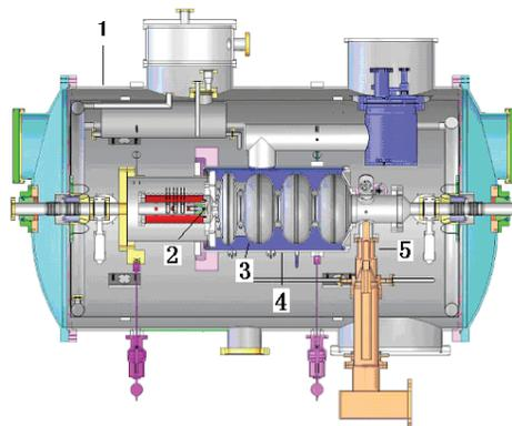
Figure 1: [1] Thermostat, [2] Photocathode (Te2Cs), [3] 3.5 cell LG Nb cavity, [4] Liquid Helium tank, [5] Main coupler
