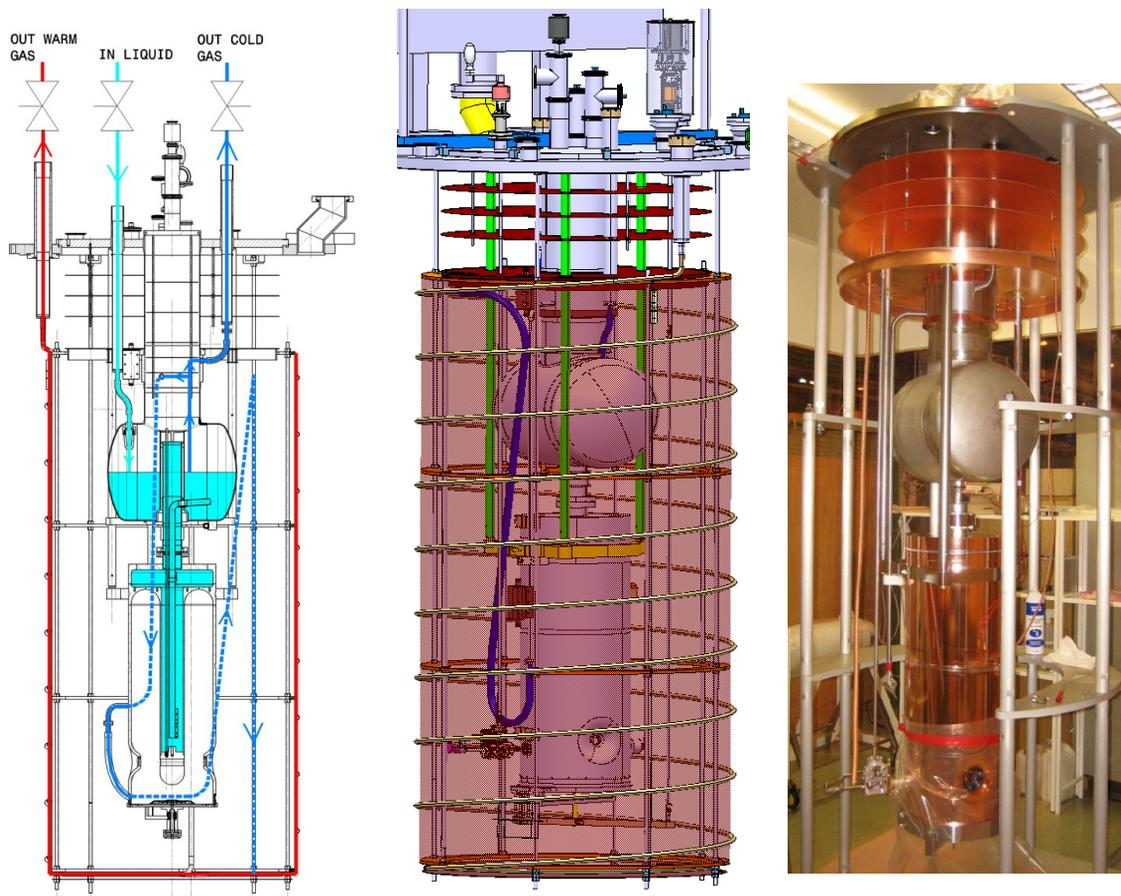
Figure 1: Cryogenic working principle, cryostat design and cryostat insert manufactured.
