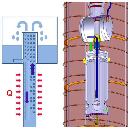
Figure 2: Thermosyphon cooling principle of the cavity.
