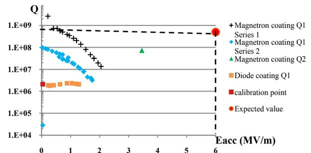
Figure 3:  $Q$  (Eacc) for different Nb coatings on copper QWR cavities. The red point is the  $Q$  value expected:  $5.10^8$  at 6 MV/m for the HIE-ISOLDE QWR cavity.
