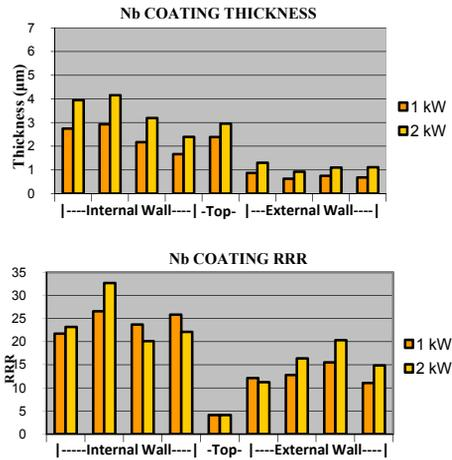
Figure 1: Thickness and RRR value obtained for coating power of 1 kW and 2 kW without cooling, on copper and quartz samples by biased magnetron (a) and diode sputtering (b).
