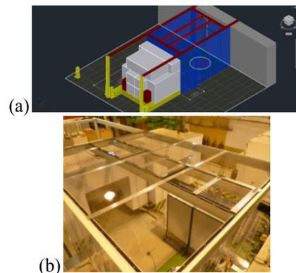
Figure 2: (a) Schematic view and (b) picture of the vertical cryostat area with the clean space for HIE-ISOLDE RF test at CERN.
