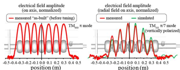
Figure 2: Typical result of an “as-built” flat fundamental mode and symmetric  $TM_{111}$ -like  $\pi/7$  HOM field profile.
