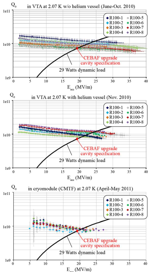
Figure 4: *R100* cavity RF performances in the VTA w/o HV (top), with HV (mid) and in the cryomodule (bottom).
