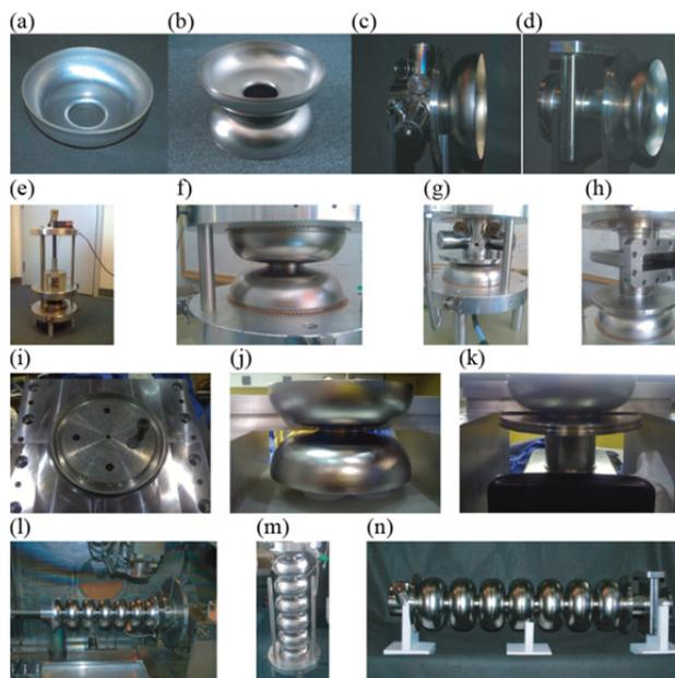
Figure 1: *R100* cavity fabrication sequence (cf. text).
