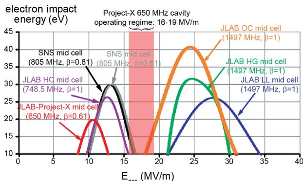
Figure 2: Electron impact energy for stable multipacting trajectories in various inner cavity cells.
