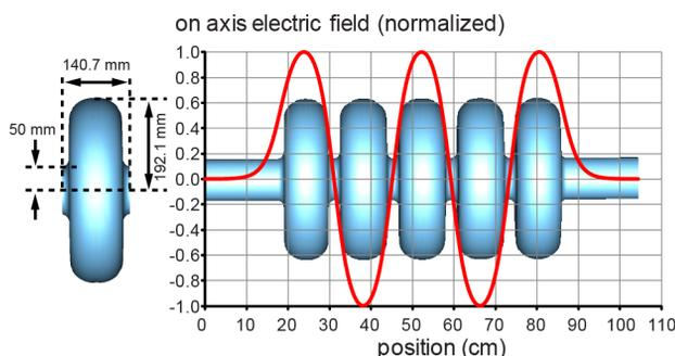
Figure 1: Medium-beta ( $\beta = 0.61$ ) 650 MHz cavity mid cell layout (left) and five-cell cavity design (right).
