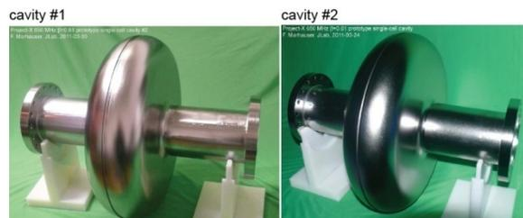
Figure 3: Medium-beta 650 MHz SRF cavities.
