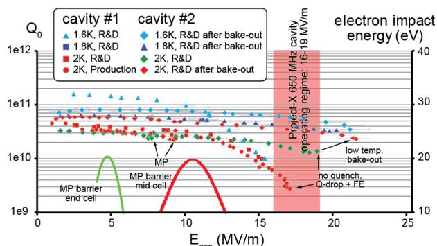
Figure 4: Unloaded quality factor versus effective accelerating field for cavity #1 and #2 respectively.
