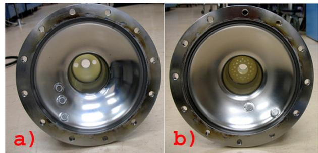
Figure 5: Photo of the new demountable cavity after treated by BEP. a) Upper half cell. b) Lower half cell.
