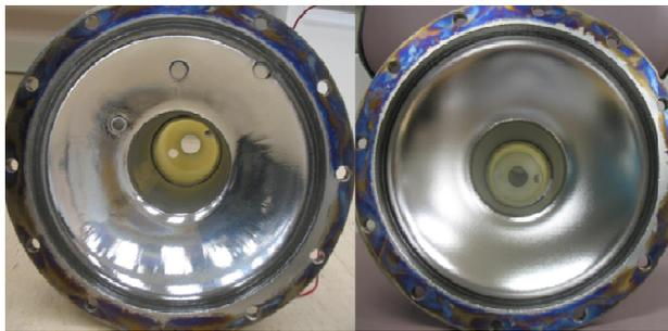
Figure 2: Photo of the demountable cavity treated by the optimized cathode shown in Fig.1a). Left is the upper half cell. Right is the lower cell.
