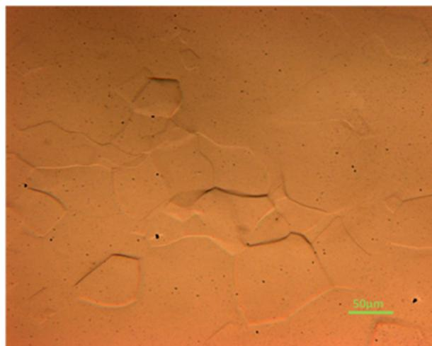
Figure 4: Typical MOM photo of the button sample that shows a Nb removal rate of  $9.7$   $\mu\text{m}/\text{min}$ .
