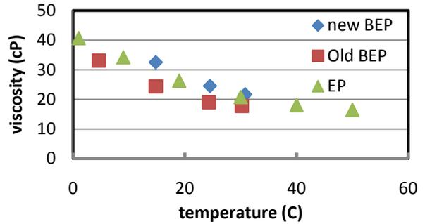
Figure 6: Viscosity measured as a function of temperature for old and new BEP and EP electrolytes.
