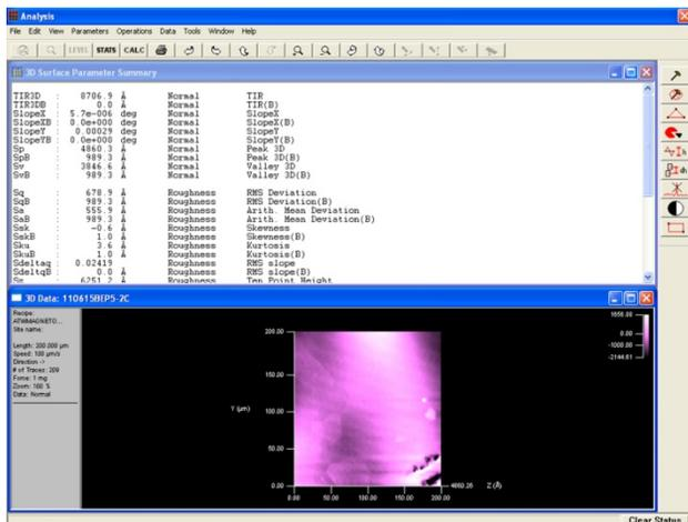
Figure 5: Profiler image of the button sample that shows a Nb removal rate of 9.7 μm/min. As shown in the upper part, the RMS of the surface is 67.9 nm.
