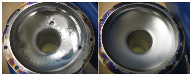
Figure 3: Photos of the demountable cavity after BEP treatment. Left is the upper cell. Right is the lower cell (see text for more details).
