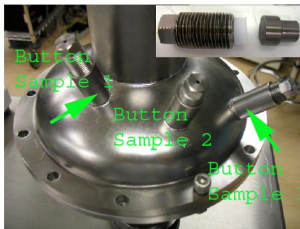
Figure 1: Photo of the demountable cavity fabricated at JLab. The arrows indicate the three button samples. The insert on the upper right corner shows the button sample assembly.
