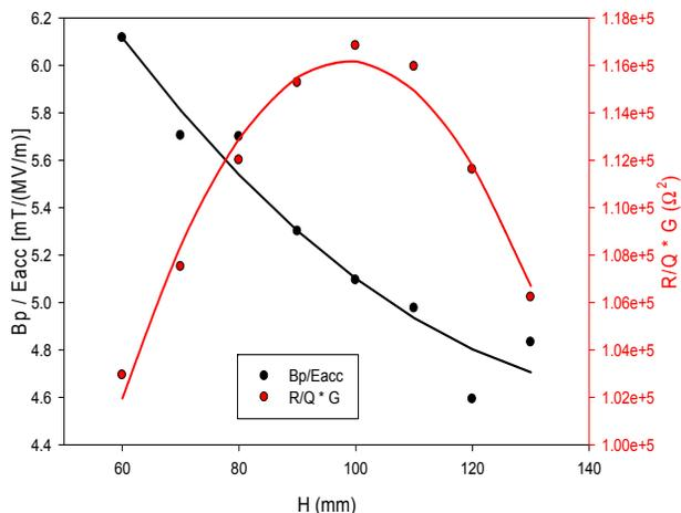
Figure 3: Normalized surface magnetic field and R/Q\*G vs. H.
