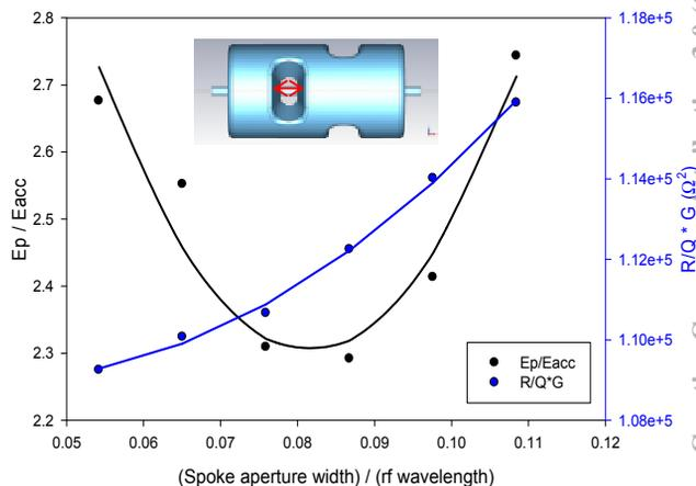
Figure 5: Normalized electric fields and R/Q\*G vs. the spoke aperture width normalized to the rf wavelength.
