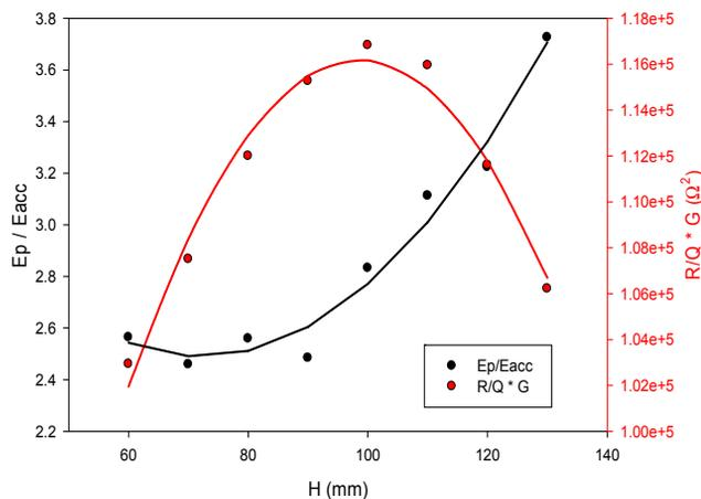
Figure 4: Normalized electric fields and R/Q\*G vs. the parameter H.
