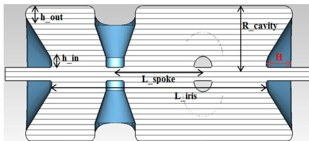
Figure 1: CST MWS cut-away view of the two-spoke 325 MHz,  $\beta_0 = 1$  cavity.
