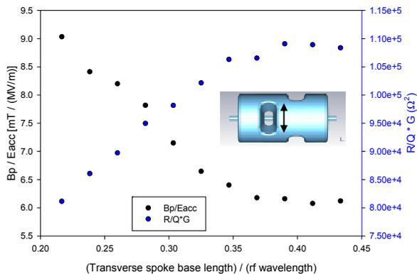
Figure 2: Normalized surface magnetic field and R/Q \* G as a function of the transverse spoke base length.
