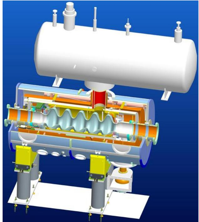
Figure 1: Schematic of BNL1 cavities immersed in helium tank (below) and connected to the ballast tank (above).
