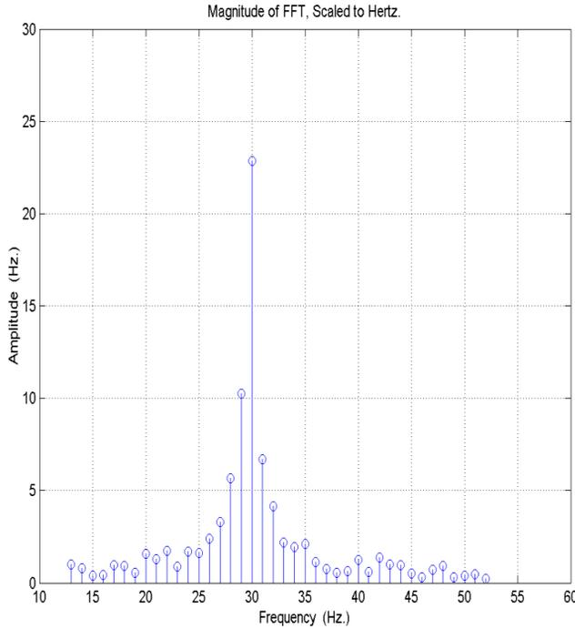
Figure 2: Onset of resonance near the 30 Hz line.
