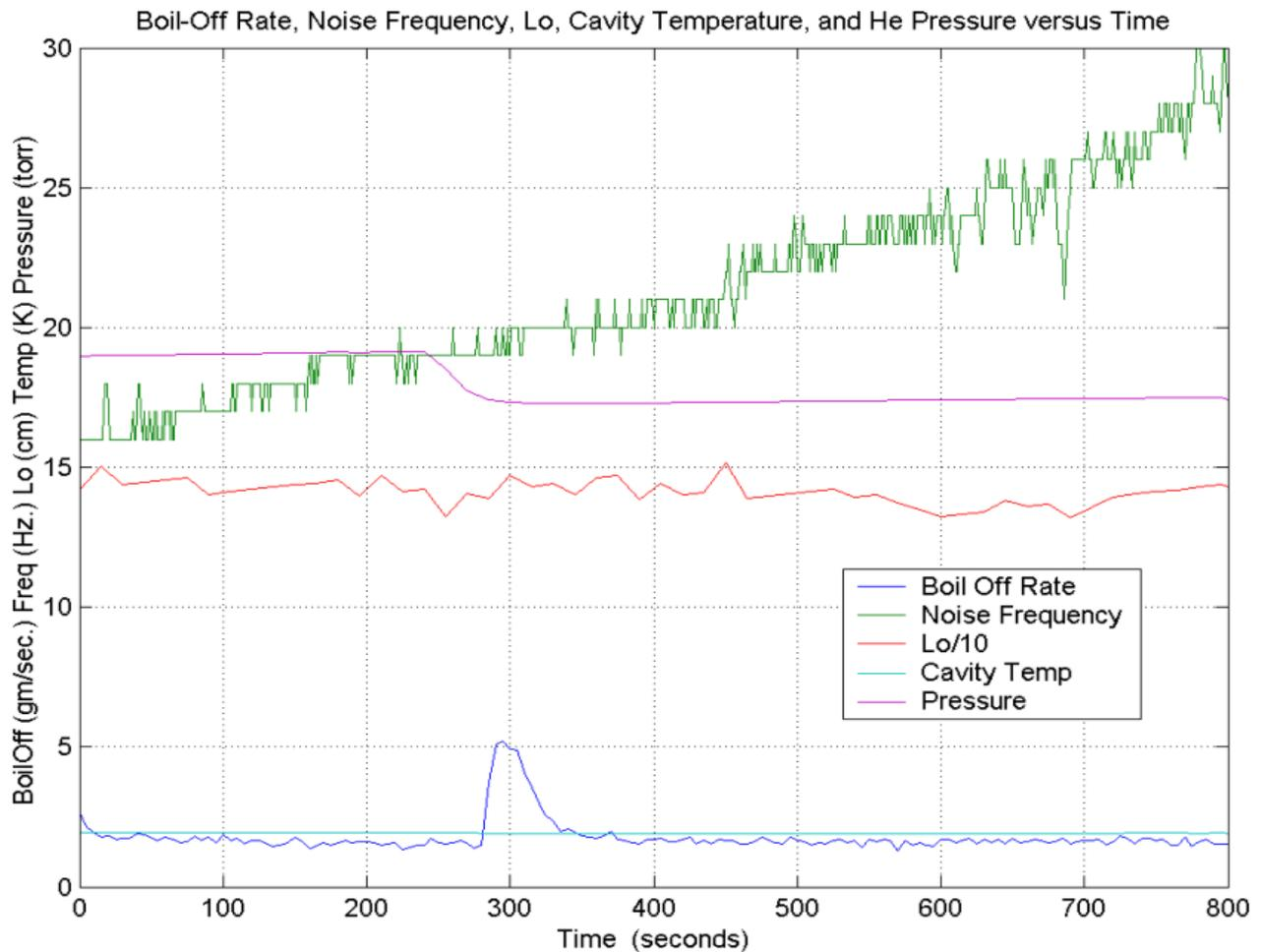
Figure 4: Change in boil-off rate, noise frequency,  $L_0$ , cavity temperature and helium pressure as a function of time.
