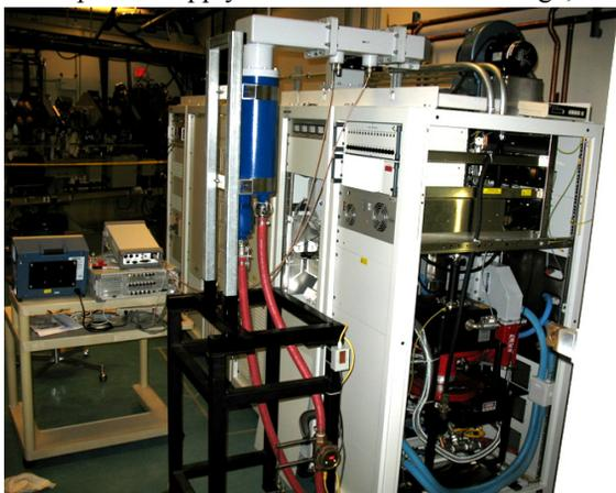
Figure 3: Photograph of the IOT Transmitter
