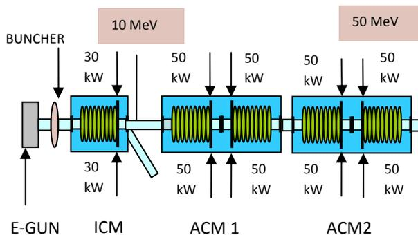
Figure 1: Basic layout of the E-linac
