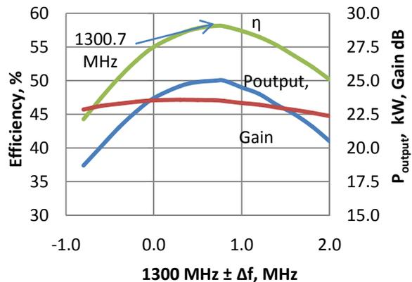
Figure 4: RF measurements of 30 kW IOT s/n 001
