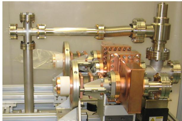
Figure 6: Coupler test stand - two CPI 65 kW coupler cold windows are mounted on a waveguide box
