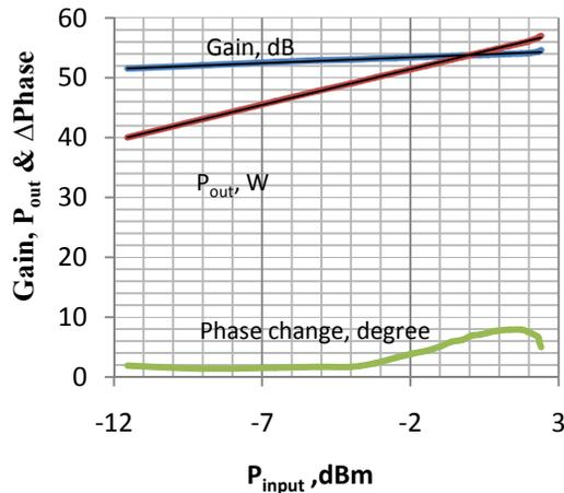
Figure 2: Measured rf characteristic of the solid state buncher amplifier
