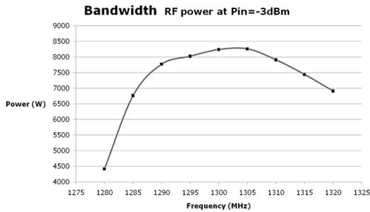
Figure 10: Bandwidth of the SSPA
