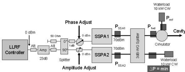
Figure 11: Setup to operate two SSPA in parallel
