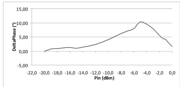
Figure 8: Phase deviation of the SSPA
