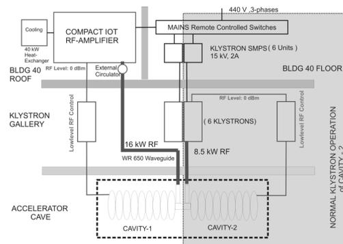
Figure 2: Block diagram of the IOT operation
