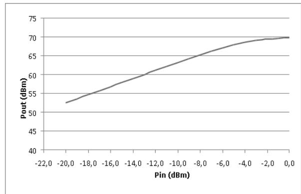
Figure 6: Gain response of the SSPA
