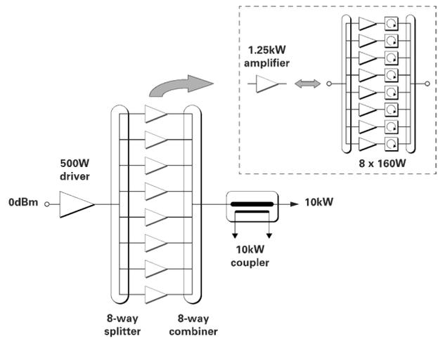
Figure 5: Block diagram of the RF-part
