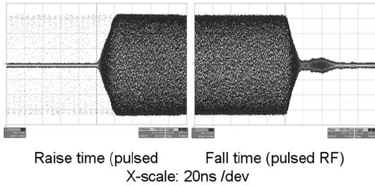
Figure 9: Raise time (using pulsed operation) (rise time 20ns, fall time 60ns resp.)
