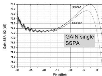
Figure 12: Individual gain curves of both SSPA
