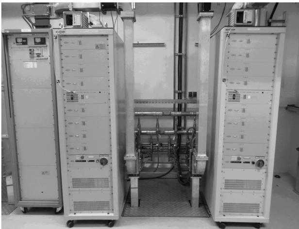
Figure 4: 10 kW SSPA (BRUKER)
