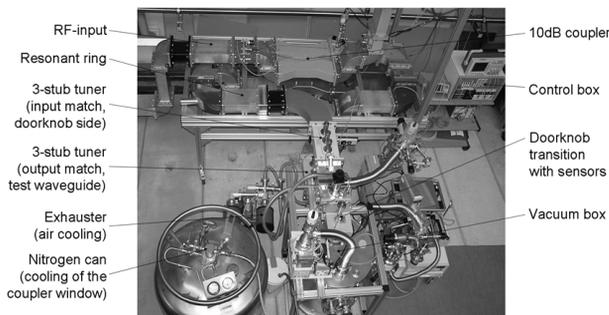
Figure 1: Layout of the resonant ring
