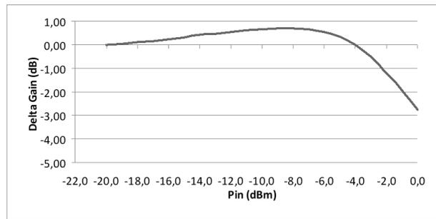
Figure 7: Gain deviation of the SSPA
