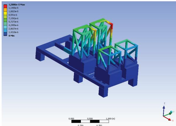
Figure 2: Main Platform Vibration Analysis
