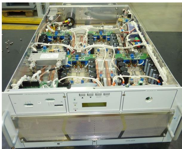
Figure 2: 7 kW amplifier unit.
