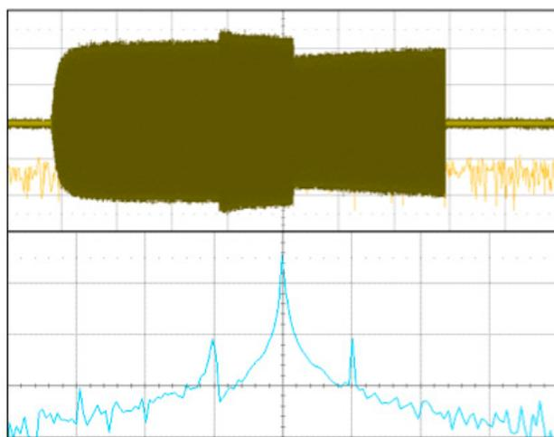
Figure 4: Top: Pulse with instability (100  $\mu$ s per div). Bottom: Spectrum with side lobes (center 352.2 MHz, span 22.8 MHz and 14.4 dB per div).
