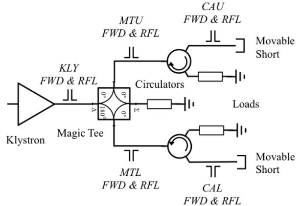
Figure 1: Test-place configuration.
