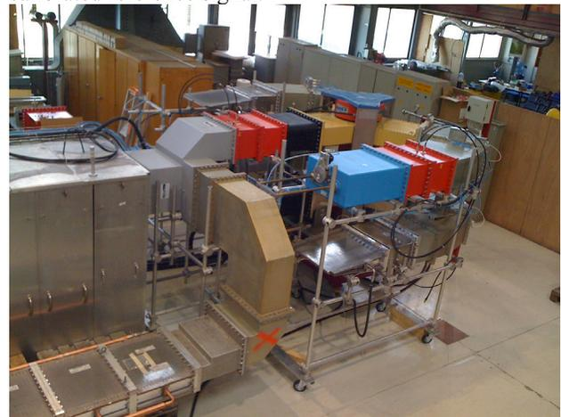
Figure 2: Linac4 test-place featuring power splitting by means of a folded magic tee (grey), two LEP circulators, two movable shorts (blue) and directional couplers for power measurements (red). The third port of the magic tee is equipped with an LHC load (bottom left).
