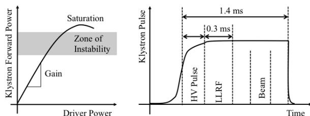
Figure 3: Klystron saturation curve & pulse envelope.
