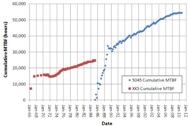
Figure 1: Cumulative MTBF for the 5045 and XK5 Klystrons.
