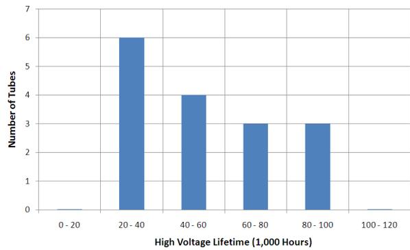
Figure 7: Lifetime of Tubes Failed for an End of Life Cathode During the Last 5 Years.
