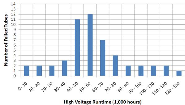
Figure 8: Lifetime of Tubes Failed for Leaky or Broken Windows Since ~1993.
