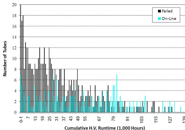
Figure 4: 5045 Cumulative High Voltage Runtime Hours.
