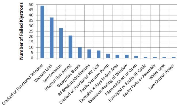
Figure 6: Reasons for 5045 Failure Since ~1993 as Determined Prior to Tube Autopsy.
