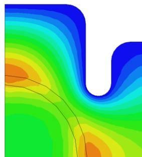
Figure 7: Output Cell Width is Used to Optimize Field Flatness in the Output Cell.
