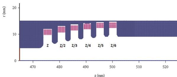
Figure 5: 6-Cell Tapered Impedance Design in MAGIC2D.
