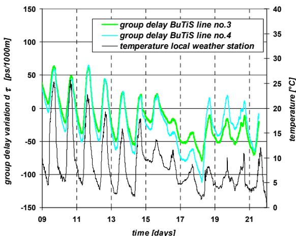
Figure 2: Group delay variation of the 1km FOC installation versus time (double passage measurement October 2010).
