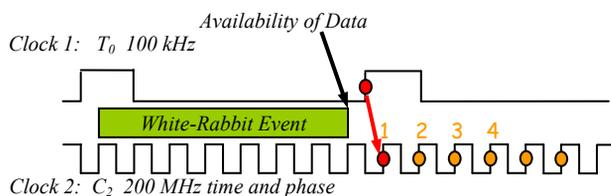
Figure 4: BuTiS method of resynchronization
