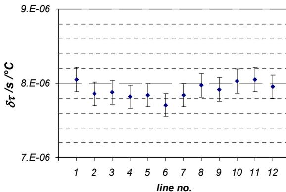
Figure 3: Difference of temperature coefficients of different fibers in a loose tube jelly filled FOC.
