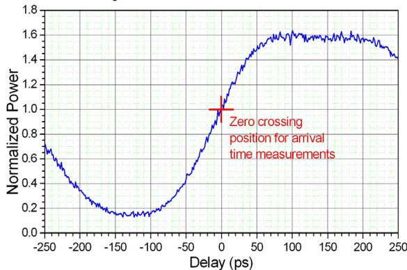
Figure 5: Beam arrival monitor characterisation showing 26 ps/dB sensitivity when operating at 40 pC bunch charge.
