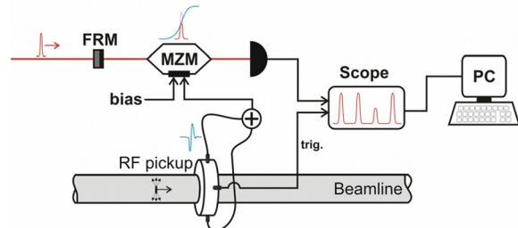
Figure 4: Concept of the beam arrival monitor.
