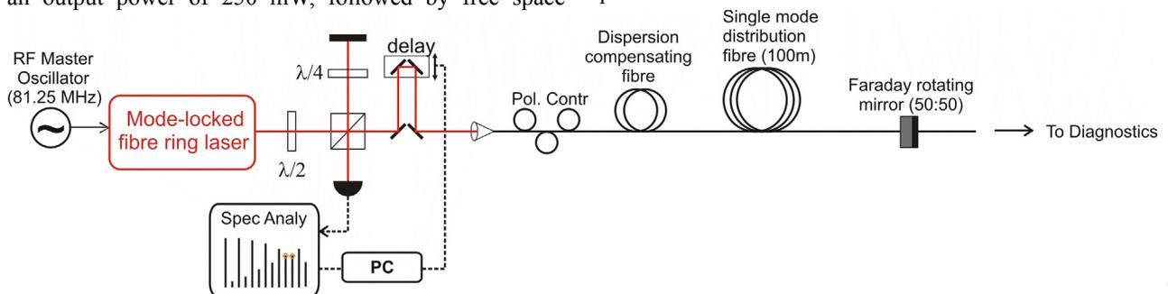
Figure 1: Layout of the optical timing scheme.
