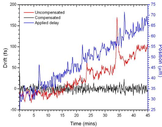
Figure 2: Measured drift of the optical link with and without the RF stabilisation scheme.
