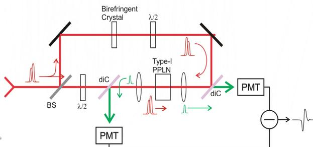
Figure 3: Configuration of the optical cross correlator based on a type-I PPLN. BS: nonpolarising beamsplitter, diC: dichroic mirror.
