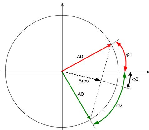
Figure 1: Principle of out phasing control.
