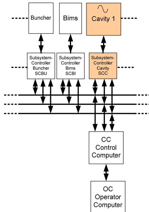
Figure 2: Concept of distributed control system.
