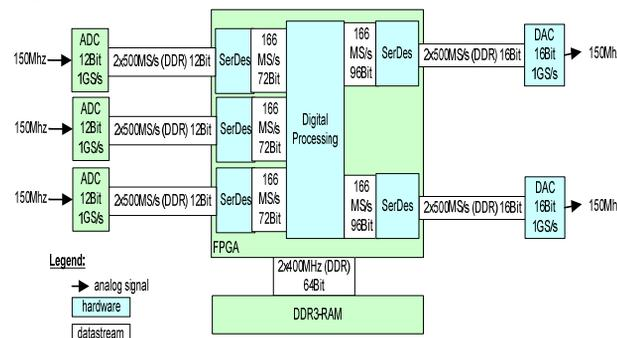
Figure 5: Dataflow on SCCRT.
