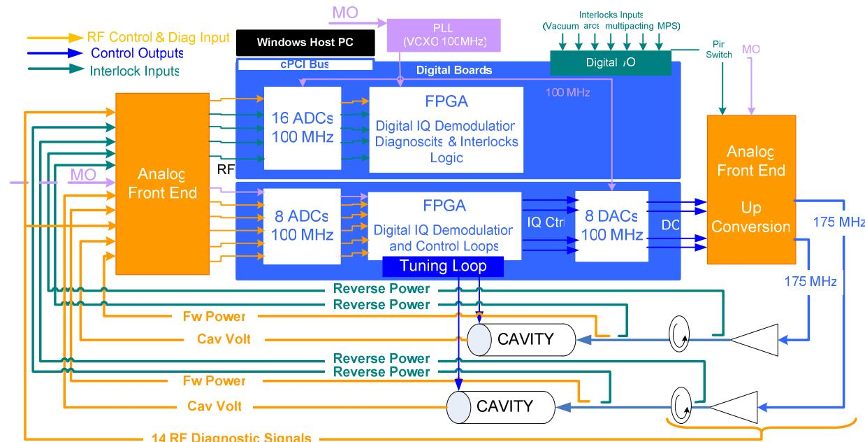
Figure 1: LLRF Hardware and Signals.
