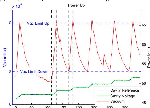
Figure 4: Automatic Conditioning of ALBA Dampy Cav.
