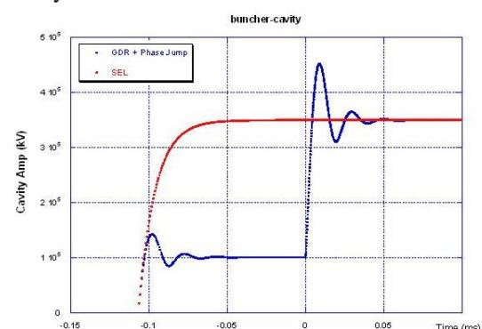
Figure 2: Cavity Voltage Amplitude with and without frequency tuning modulation during cavity filling.
