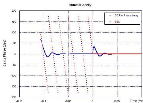
Figure 3: Cavity Voltage Phase with and without frequency tuning modulation during cavity filling.
