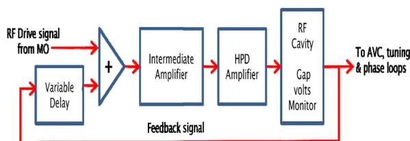
Figure 3: RF feedback system diagram.
