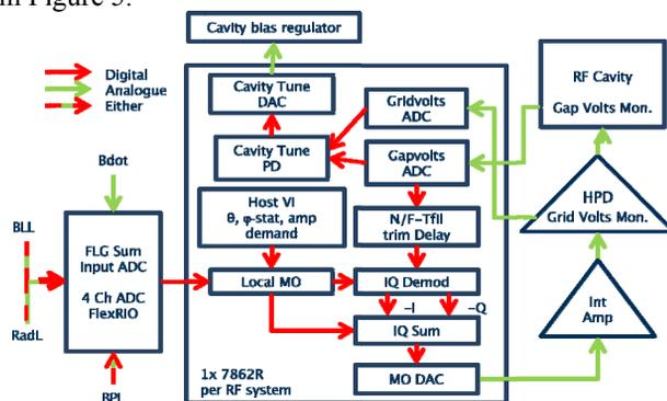
Figure 5: System diagram for a digital local oscillator.
