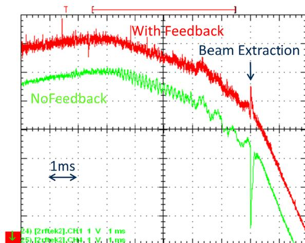
Figure 4: Gap voltage envelopes for RF feedback loop.
