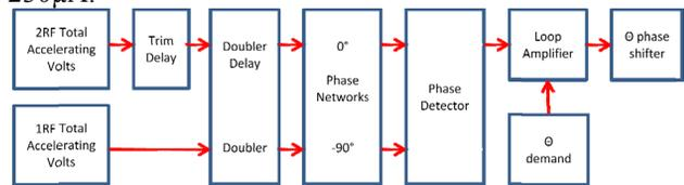
Figure 2: Closed loop for  $\theta$  control.
