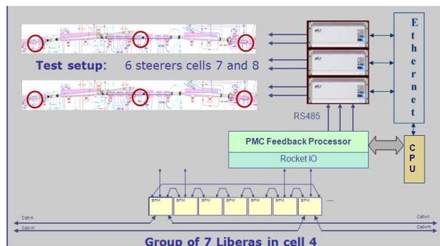
Figure 3: layout of the partial setup adopted for the tests.
