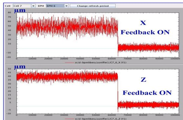
Figure 4: BPM signals with orbit correction OFF (left part) and ON (right). H scale = 10s of record, V scale = 10μm/div.
