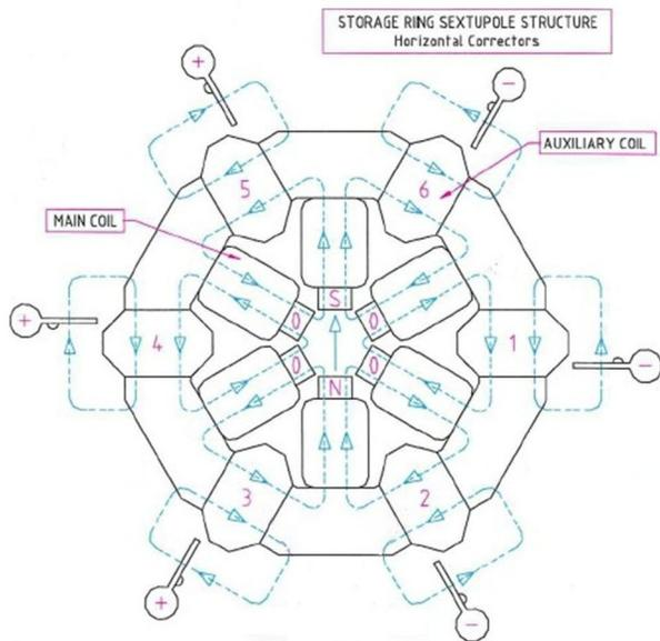
Figure 2: layout of the auxiliary correctors in a sextupole.
