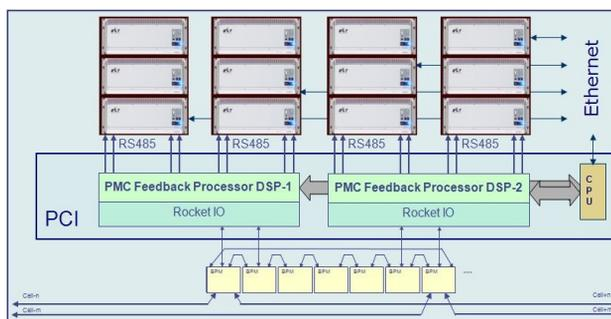
Figure 1: layout for 1/4<sup>th</sup> of the system connected to the Libera BPMs of one of the 32 cells.
