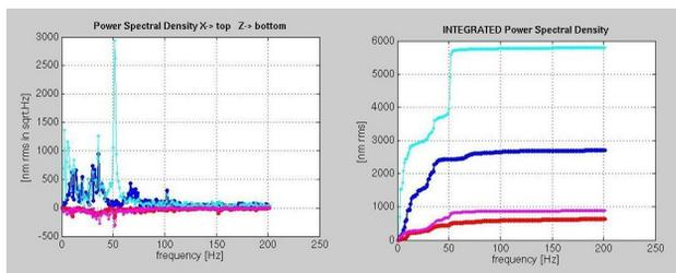
Figure 5: Power spectral density (left) and integrated power spectral density (right) averaged over the BPMs of the 2 corrected cells with and without orbit correction. Light blue, dark blue: H signals, purple, red: V signals.
