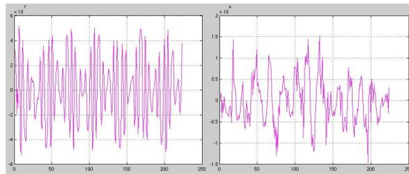
Figure 7: Horizontal (left plot) and vertical (right plot) response of the beam to a horizontal kick of 150nrad.
