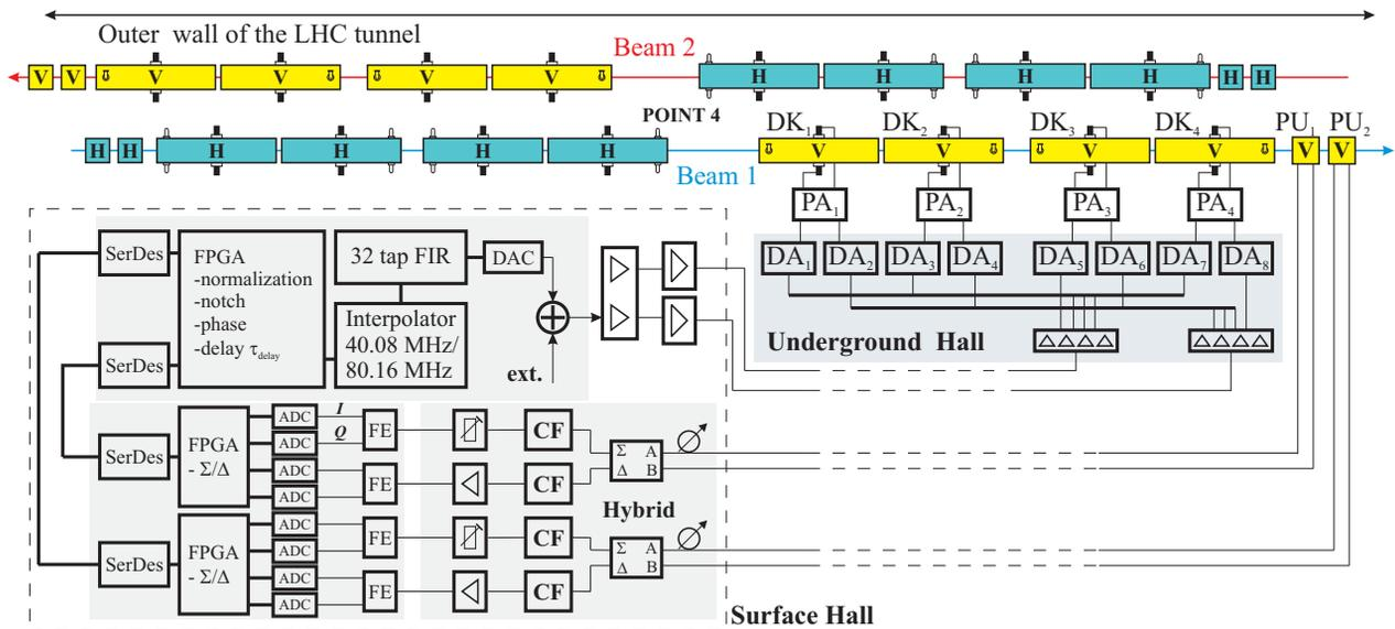
Figure 1: Block diagram of transverse damper system, reproduced from [3, 4].
