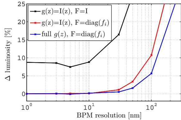
Figure 3: The graphs show, how different controller variants (full  $g(z)$  means  $g = I(z)T(z)P(z)L(z)$ ) influence the luminosity loss due to the BPM resolution.
