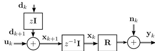
Figure 1: Block diagram of the model describing the beam oscillations in the ML and BDS. The unity matrix is symbolised by  $I$ . The details are explained in the text.
