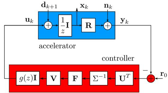
Figure 2: Block diagram of the trajectory feedback system. The coefficients  $f_i$  are collected in the diagonal matrix  $\mathbf{F}$ . The normalisation of the loop gains is achieved by the multiplication with  $\mathbf{\Sigma}^{-1}$ .
