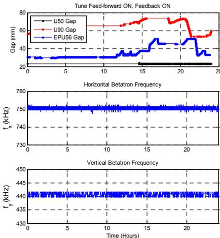
Figure 7: Tune keeps constant when feedback loop is closed.
