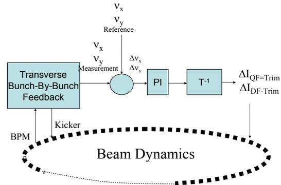
Figure 4: Functional block diagram of the tune feedback experiment.
