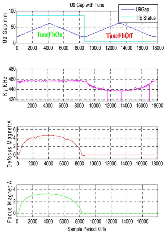
Figure 5: Vertical tune status corresponding to undulator U9 gap without and with tune feedback. Unstable beam and tune measurement fail when U9 gap is operated.
