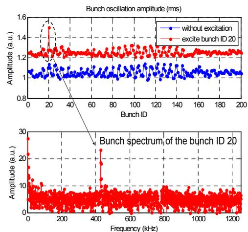
Figure 1: Tune measurement by single bunch excitation and Fourier analysis of its small bunch oscillation.
