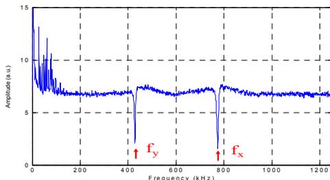
Figure 2: Tune measurement by the notches occurred in the bunch averaged spectrum due to negative feedback natural of the transverse feedback loop.
