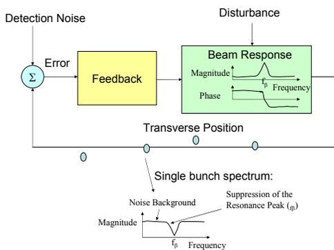
Figure 3: Functional block diagram of the tune feedback experiment.
