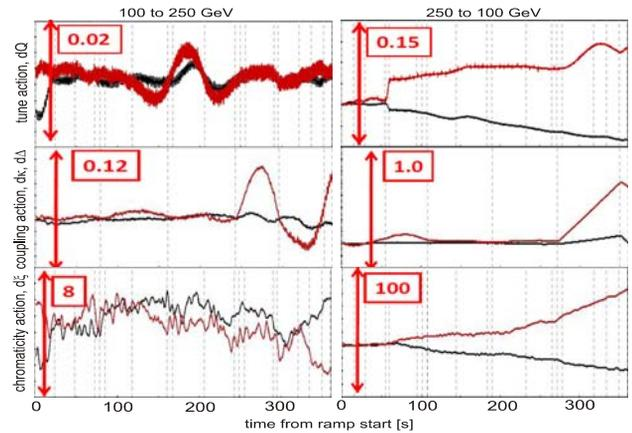
Figure 9: Action of the tune (top), coupling (middle) and chromaticity (bottom) feedback loops in the yellow ring.
