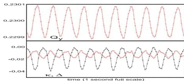
Figure 2: Vertical tune ( $Q_y$ , top) and coupling coefficients ( $\kappa$  and  $\Delta$ , bottom) measured at store without feedback.
