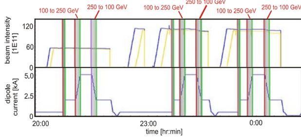
Figure 7: Beam intensities (top) and dipole current (bottom) during 3 consecutive up-and-down ramps.
