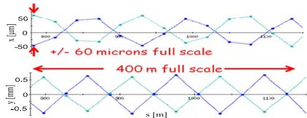
Figure 1: Horizontal ( $x$ , top) and vertical ( $y$ , bottom) difference orbit measurements in a RHIC arc.
