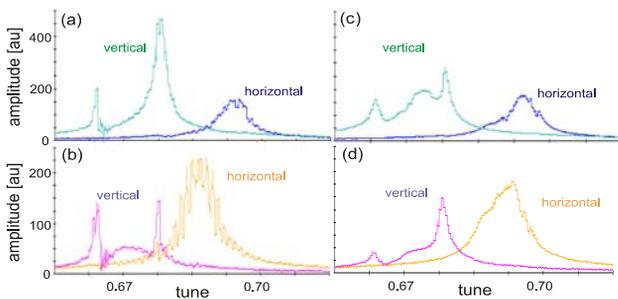
Figure 4: Measured beam transfer functions without (a,b) and with (c,d) 10 Hz feedback in the blue (a,c) and yellow (b,d) rings.
