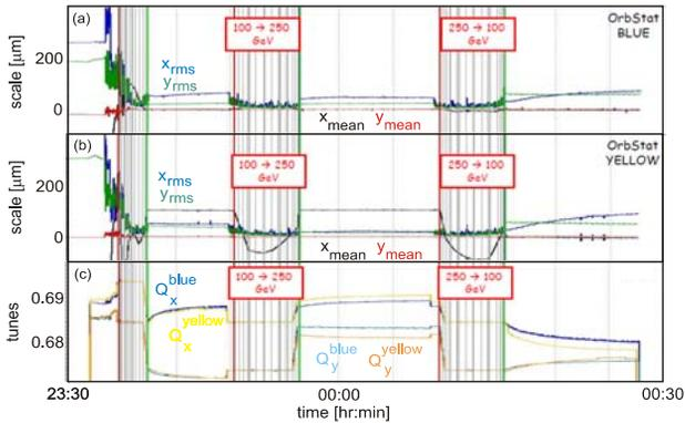
Figure 8: Beam orbit parameters (a,b) and tunes (c) during an up-and-down ramp with full beam intensities.
