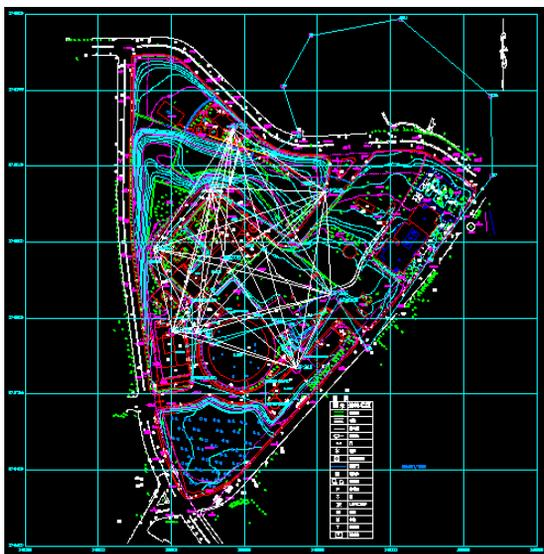
Figure 1: The NSRRC site and survey control network.
