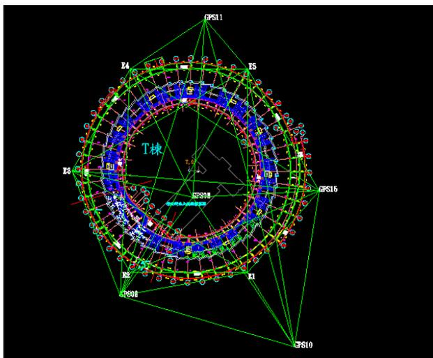
Figure 6: The control points and network survey of TPS construction
