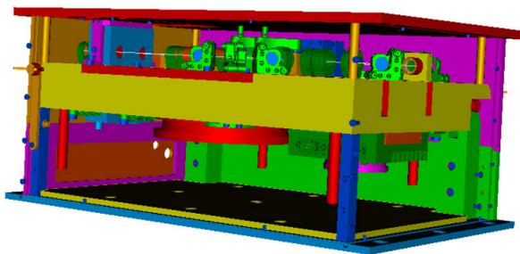
Figure 2: Design drawing of a fiber link stabilization unit.
