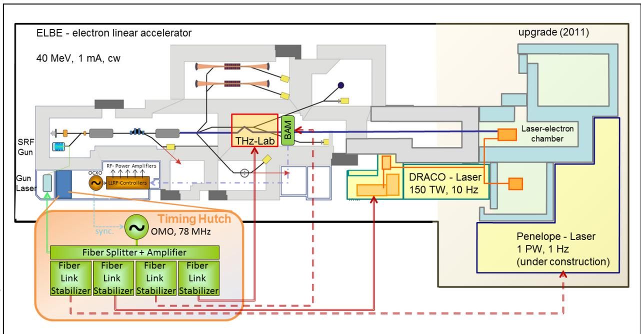
Figure 3: ELBE Layout after extension including synchronization scheme currently under construction.
