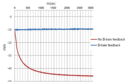
Figure 4: 400 MeV/u Carbon beam positions with and without B train feedback.
