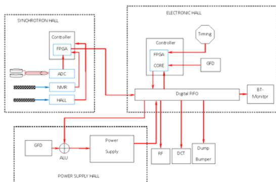
Figure 1: Layout of the B-TRAIN system.
