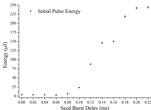
Figure 4: Energy of first amplified pulse as a function of the delay between pump and seed bursts.
