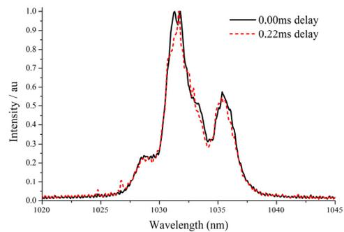
Figure 8: Amplified seed spectra for different delays between pump and seed bursts.
