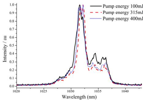
Figure 7: Amplified seed spectra for low, high and maximum pumping.
