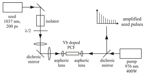
Figure 1: Experimental arrangement.
