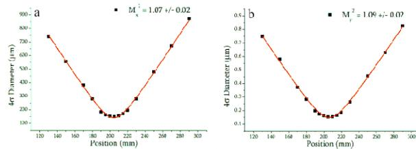
Figure 6: a)  $M_x^2$  and b)  $M_y^2$  of PCF output.
